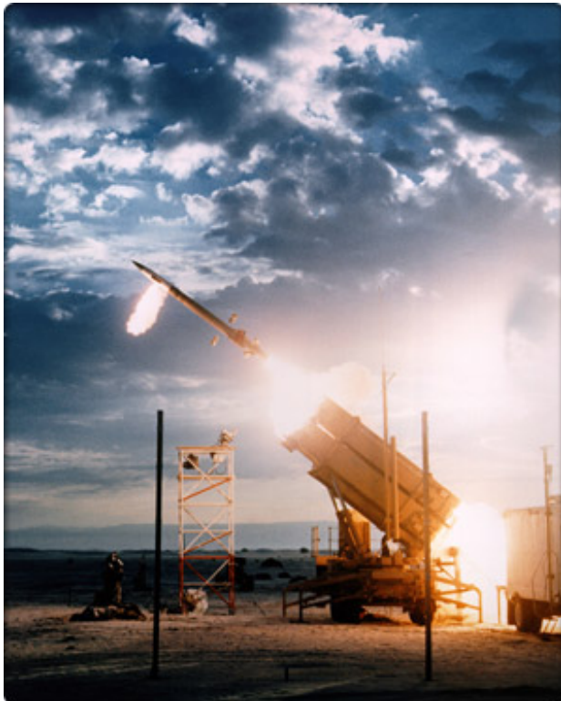
A launcher of the PAC-3 ground-based antimissile missile deployed to a Self-Defense Force base
