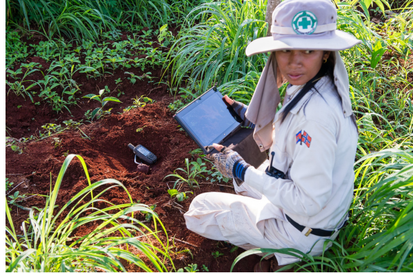
Ratanakiri Province, Cambodia, 2014 - The leader of an NPA technical survey team uses her tablet computer to record a bomblet her team has found with the precise location derived from her GPS tracker.
