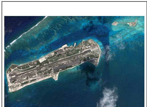
Satellite photo of Johnston Atoll, about 1,390 km (860 mi) west of Hawaii. Four islands compose the total landmass of 2.6 sq km. Johnson and Sand islands are both enlarged natural features, while Akau and Hikina are two artificial islands formed by coral dredging. Johnston Island, by far the largest, contains an airstrip. (Caption by CIA/Image by NASA)
