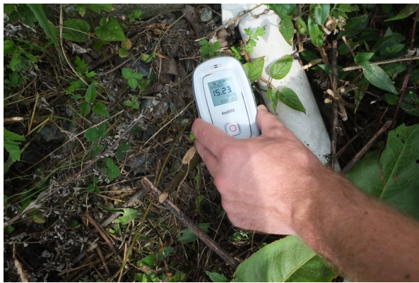
Radiation reading taken in Iitate Village, September 2013. This reading of 15.23 microsieverts per hour translates into 133.4 millisieverts a year - far above govt. limits.
