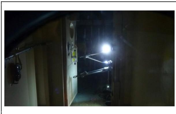
Remotely operated by TEPCO workers, at 11 a.m. that day, the PackBot entered the turbine buildings of Unit 1 and 3, then opened the double doors to go into the reactor buildings, measuring radiation levels, temperature,
