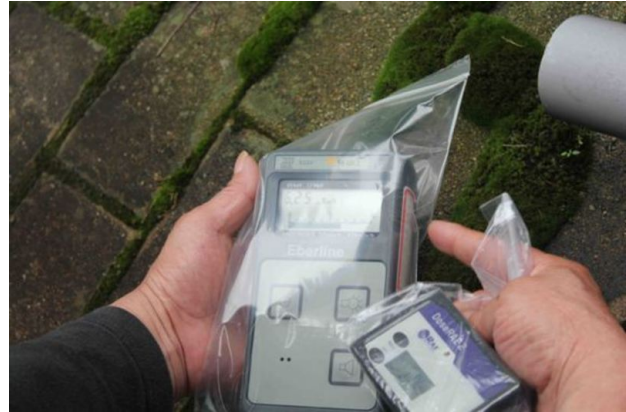
A hot spot in the suburbs of Fukushima city, August 2011: the dosimeter records 6.25 microsieverts per hour (54.75 mSv a year). (Photo: Paul Jobin)
