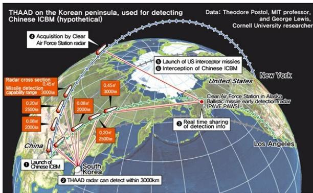
**Figure 2) A THAAD radar stationed in South Korea can be configured to track China’s ICBM’s and relay the data to a missile defense system in Alaska so that the missiles can be destroyed before reaching intended targets in the U.S.**
