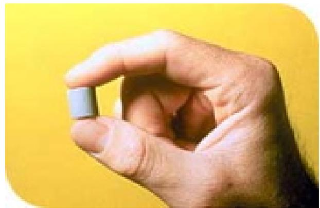
A typical pellet of uranium weighs about 7 grams (0.24 ounces). It can generate as much energy as 3.5 barrels of oil, 17,000 cubic feet of natural gas, or 1,780 pounds of coal.
