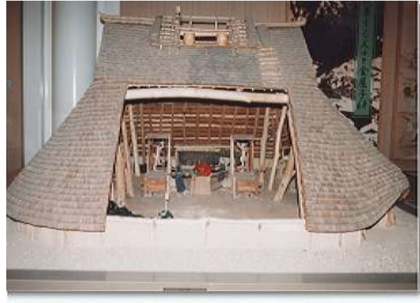
A model of a takadono, a high-roofed structure with a furnace and foot bellows (tatara), on display at Wako Museum in Shimane Prefecture.
