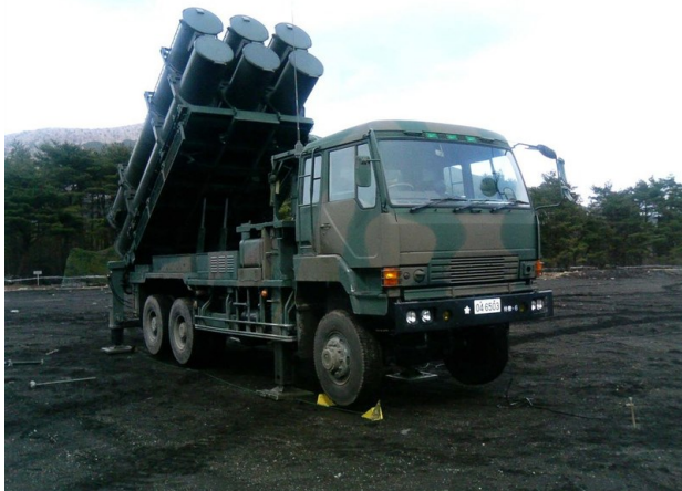
Truck carrying Type 88 missiles. Also known as SSM-1 or Shibasuta, this missile was developed by Mitsubishi Heavy Industries from the Air SDF Type 80 (ASM-1) air-to-surface anti-ship missile. 28
