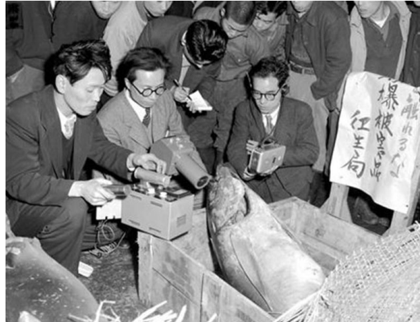
Testing tuna for radioactive contamination following the Lucky Dragon No. 5 incident
