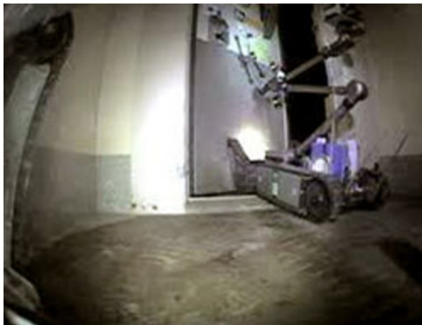
Packman: A PackBot, U.S.-made remote-controlled machine, opens a door to the main reactor building of unit 2 at the Fukushima No. 1 nuclear plant on April 18. KYODO/TEPCO
