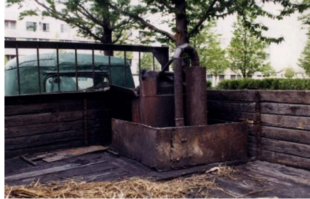
DPRK truck powered by a coal (and/ or biomass) gasifier. Source: Nautilus Institute
