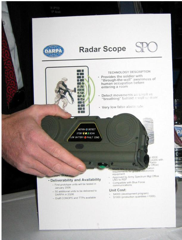
Radar Scope to sense through walls
