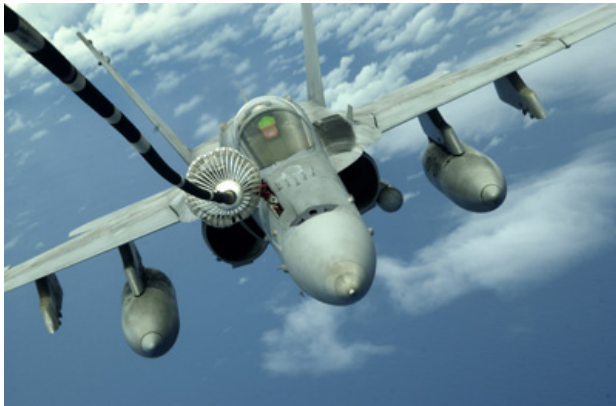
A US F/A-18D from Marine Corps Air Station Iwakuni, Japan, refuels over the Pacific Ocean from a KC-10 Extender
